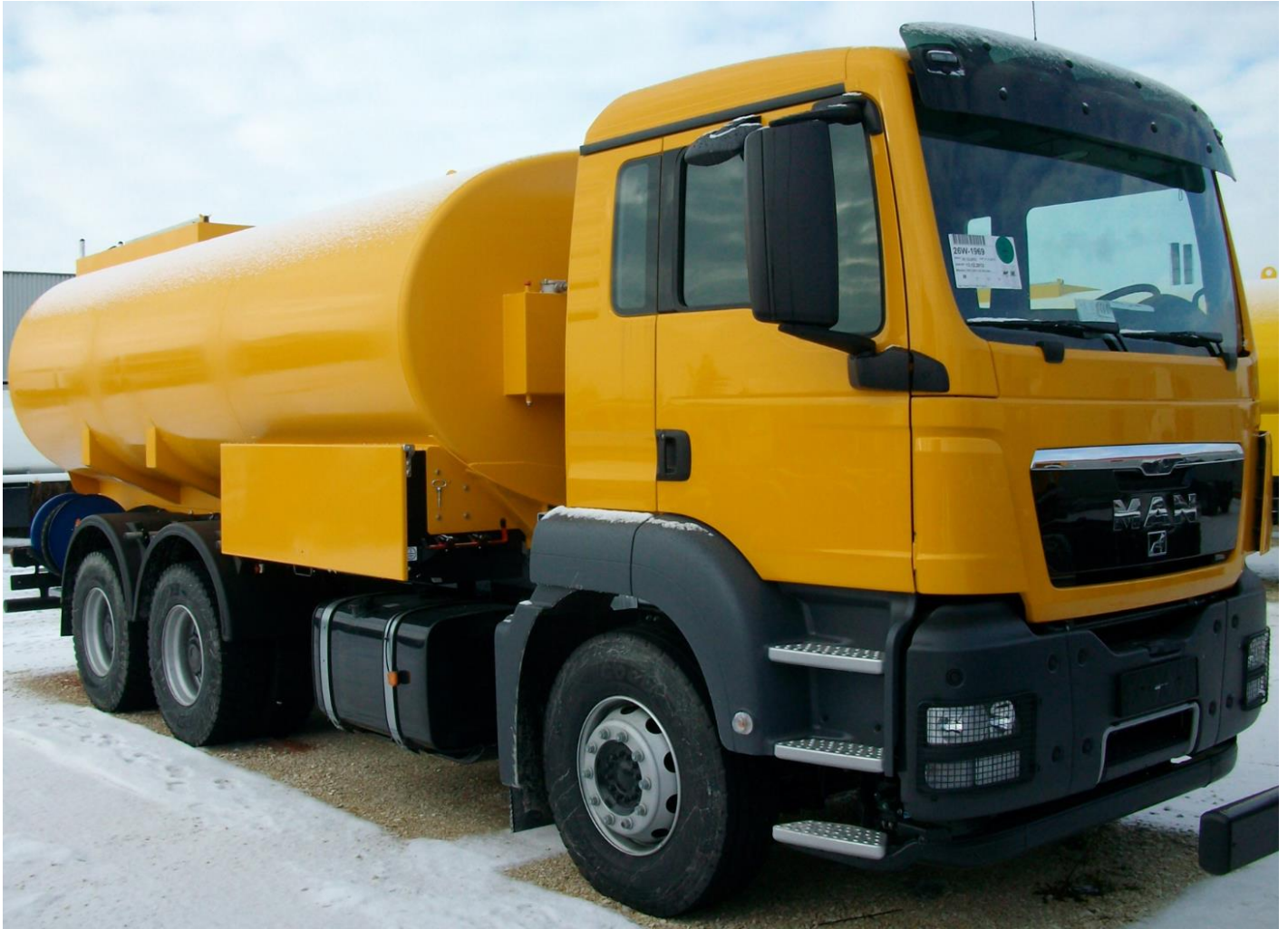
MAN TRUCK, Model: TGS 33.360 BB-WW (6X4) with diesel tank superstructure of 20.000 ltr.
