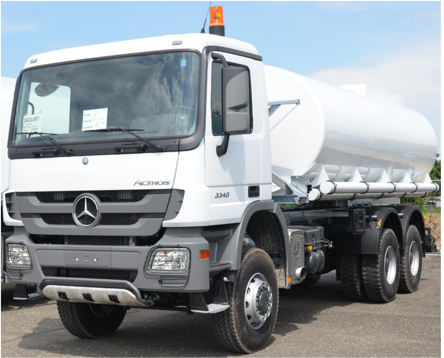
16.000 ltr. Diesel tank superstructure on Mercedes-Benz 3340 (6x6) truck
