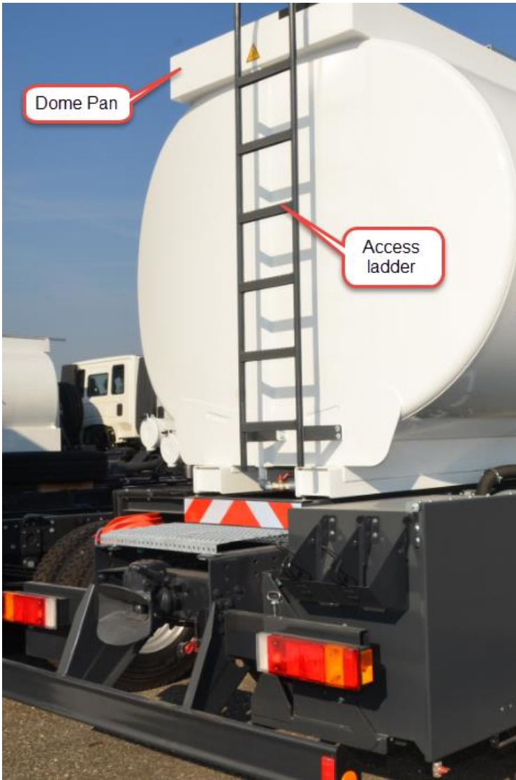
Rear view of fuel tank superstructure (Standard)
