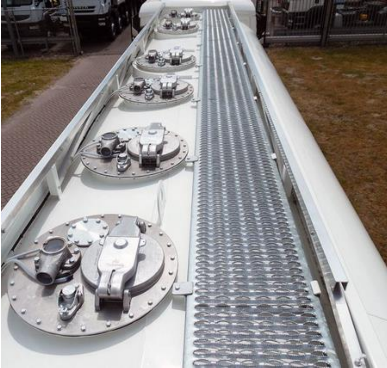
Open mesh walkway on the right-hand side of the manhole cover and collapsible handrail (safety barrier!) along the dome-pan. (Collapsible handrail in hinged position, right side) ( Standard )
