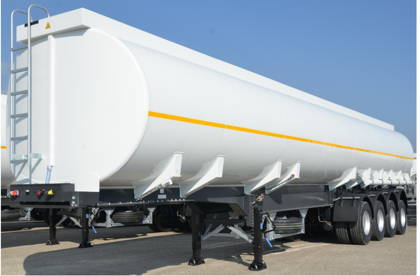
60 000 ltr. Diesel Fuel Tank Semi-Trailer with BPW axles
