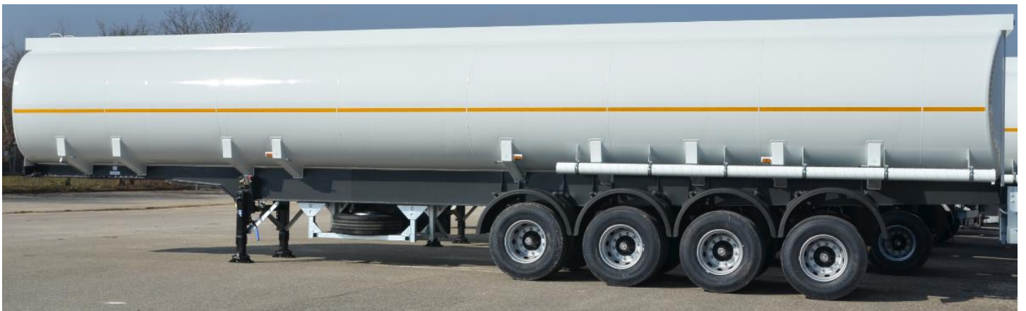
60 000 ltr. Diesel Fuel Tank Semi-Trailer with BPW axles
