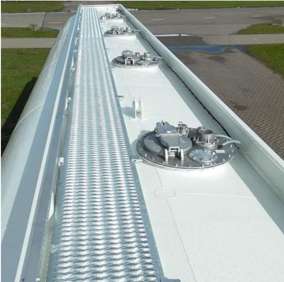
Dom pan on top of 60 000 ltr. Diesel Fuel Tank Semi-Trailer with open mesh walkway on the left-hand side of the manhole cover with collapsible handrail (safety barrier) along the dome-pan. Collapsible handrail in hinged position.
