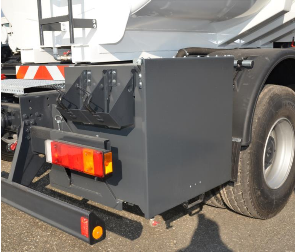
Protection box for spring loaded hose reel, 20 m hose, DN38 with fueling nozzles (Option)
