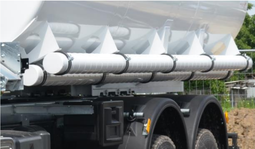
Two hose-carrier (tubes), all mounted on one side of the tank with hoses. (Standard)
