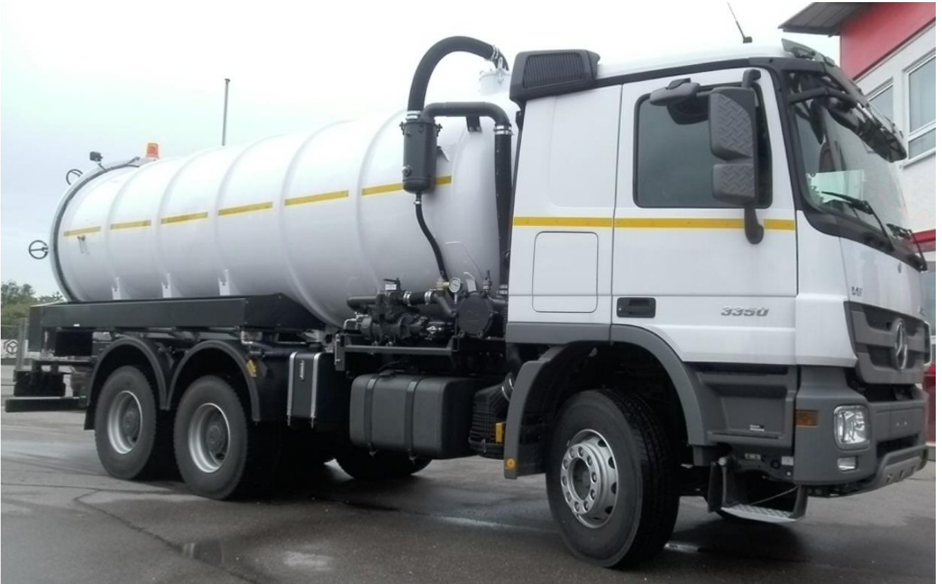
Vacuum Tank Truck 20 000 ltr. capacity
