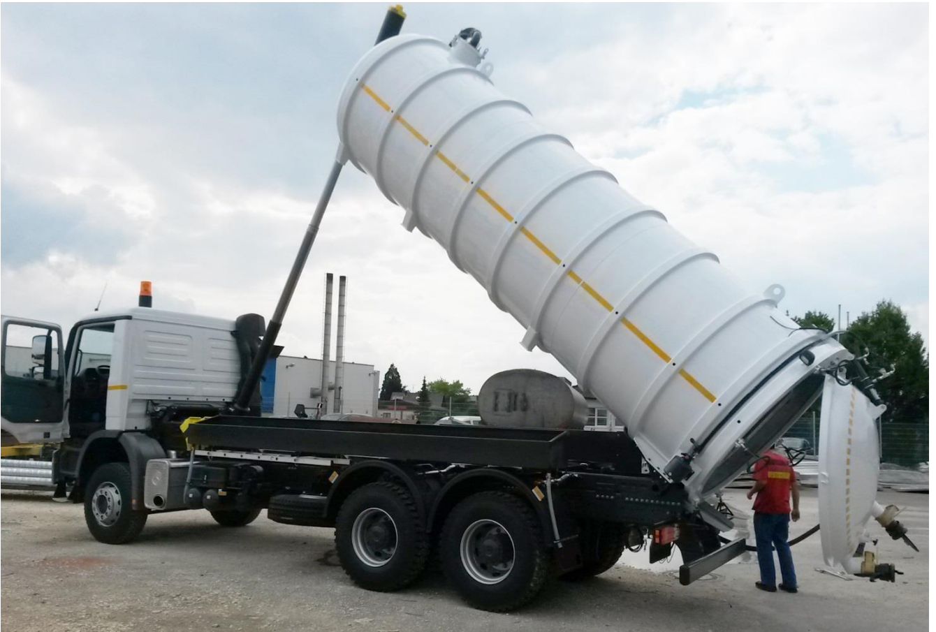
Vacuum Tank Version with Telescopic Tipping Cylinder (HYVA, Germany). Including Pneumatic Interlock System (PIS) for additional safety.
