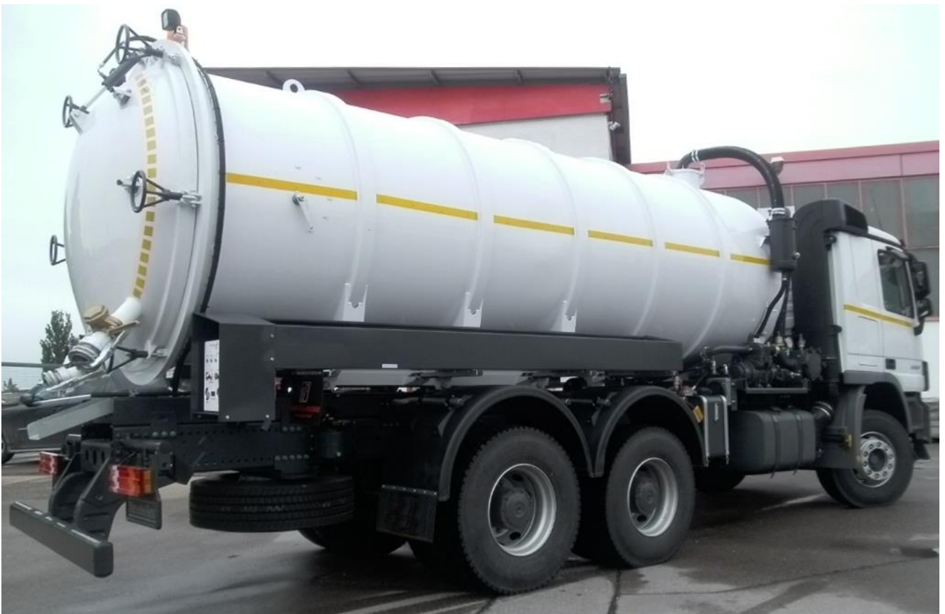
Hydraulic operated full rear opening of the vacuum tank
