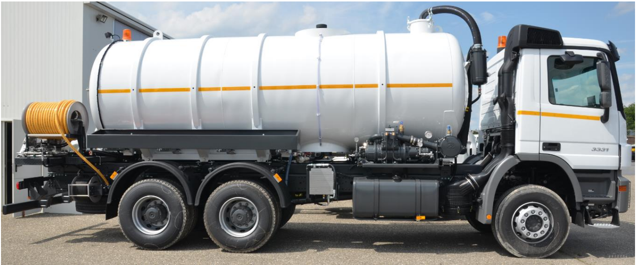
VACUUM – JETTING – FLUSHING – TANK – TRUCK. Capacity: 180000 ltr. (17 000 ltr. vacuum tank and 1 000 ltr. fresh water)
