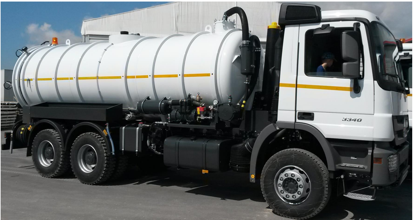
VACUUM – JETTING – TANK – TRUCK. Capacity: 18 000 ltr. (17 000 ltr. vacuum tank and 1 000 ltr. fresh water) Description on page 15
