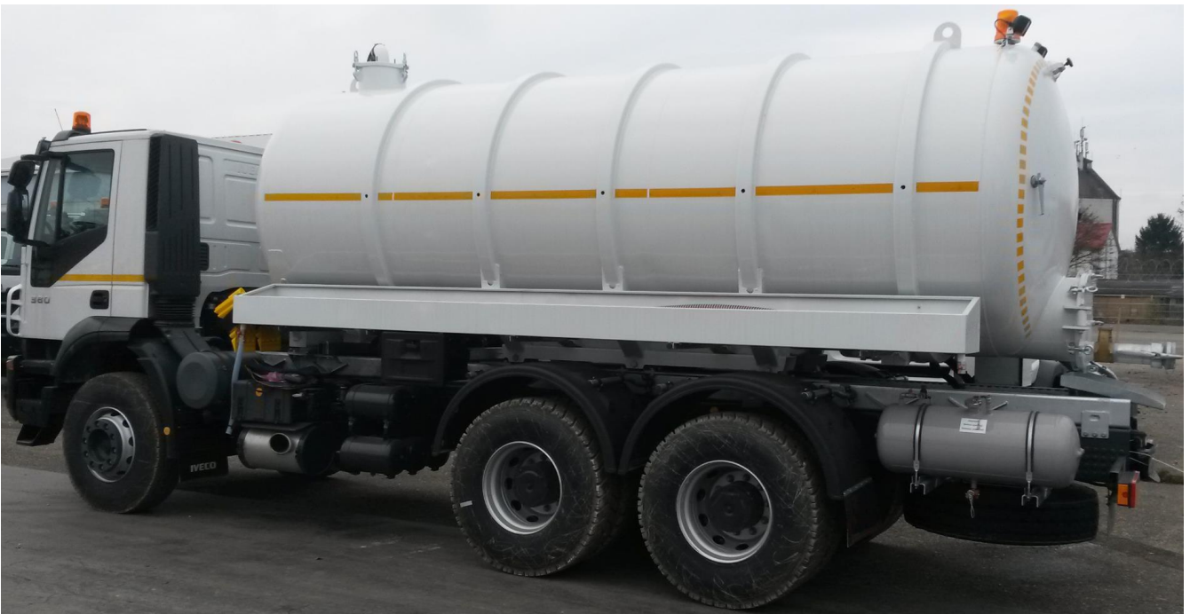
Vacuum tank truck 16 000 ltr. with small (grey) fresh water tank (120 ltr.) behind, for hand cleaning etc.
