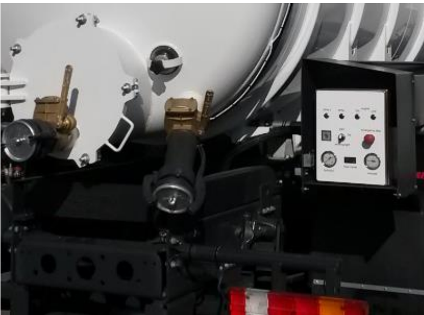
Rear view. Man hole 600 mm. Open control box on the right.
