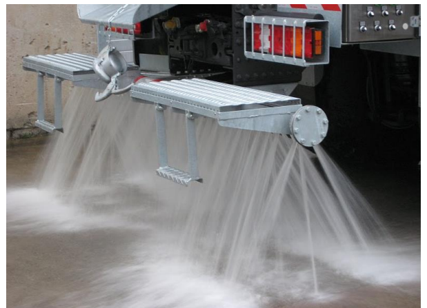
Spray bar front or/and rear (also available with adjustable nozzles)
