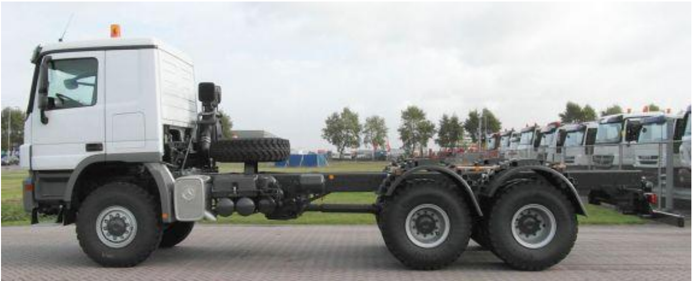
Truck chassis (6x6). Wheel base 4500 mm. M- or S-Cabin. 40 tons. Version (9/16/16 tons. axles)
