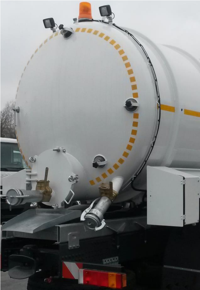
Rear view. Man hole 600 mm. Lockable control box (white color) on the right. Rotating beacon and two working lights. Subframe hot-dip galvanized.
